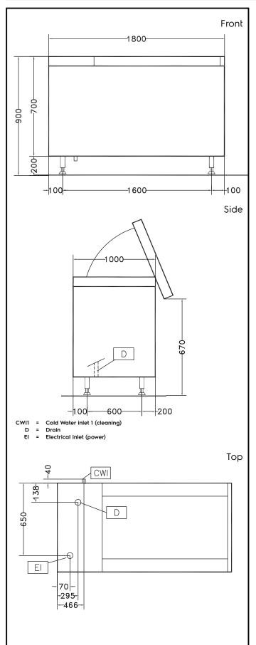
**Electric Total Watts:** 660036 (LV500R) 1.6 kW **Key Information:** Usable well capacity: 500 It Load per cycle - light vegetables: 14 kg Load per cycle - heavy 70 kg vegetables: 1800 mm External dimensions, Width: External dimensions, Depth: 1000 mm External dimensions, Height: 850 mm
